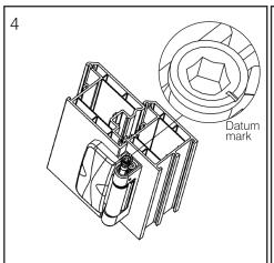
Offer sash to frame and insert hinge pin with datum mark away from sash, as shown above.
