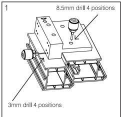
Ensure jig is orientated correctly - the top of the jig should be positioned towards the top of door, as shown above.
