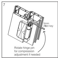
Fine compression adjustment is achieved with a 5mm Allen key and rotating the hinge pin 90 degrees, as shown above.
