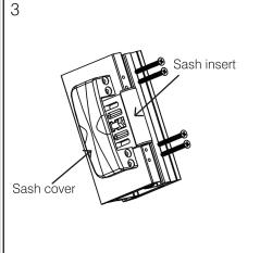
Ensure sash insert (shown above) is orientated correctly - dependent on sash over-rebate height. Recommended screw size is 4.2 x 42mm drill point bugle head (part no. 136630)
