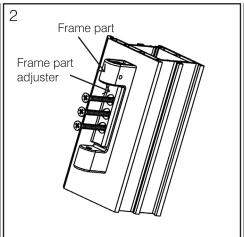
Ensure frame part adjuster is positioned to the top of the frame part as shown above. Recommended screw size is 4.2 x 42mm drill point bugle head (part no. 136630)
