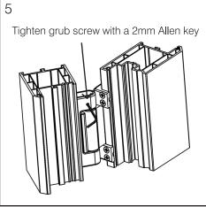
Tighten grub screw onto hinge pin with 2mm Allen key to secure, as shown above.
