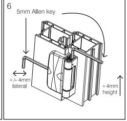
Adjustment is achieved by inserting a 5mm Allen key, as shown above.
