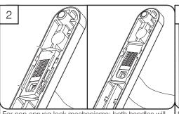
For non-sprung lock mechanisms; both handles will require the supplied spring cassette to be fitted. As shown above, align the spring cassette at an angle and then push firmly until located.
