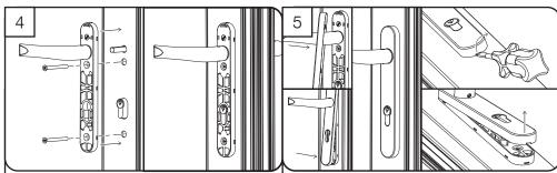
Slide the internal backplate onto the spindle and up to the internal side of the door. Select the correct length screws (supplied). Insert both screws and screw together taking care not to over tighten.
