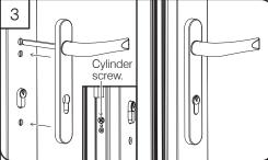
Slacken off the cylinder screw. Insert correct length of spindle (supplied) into the external lever. Slide the spindle through the lock mechanism from the external side of the door. Postion the external backplate up against the door, clearing the cylinder.
