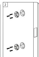
Using the screws provided, screw 'fitting A' to the door where you have marked, one on the top marking and one on the bottom. make sure it is secure.
