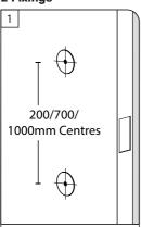
Suitably line the holes up on 'Fitting A' to where the handle will be fitted on the door,
