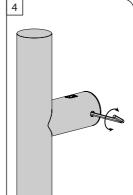
Tighten the grub screws at the top and bottom fixing the handle to 'Fitting A'.
